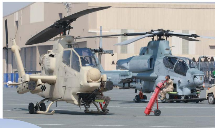
Top: Two different generations of AH-1 Cobras. On the left is the upgraded 1960s era AH-1FB and on the right, the 2020s five-bladed AH-1Z Zulu.
