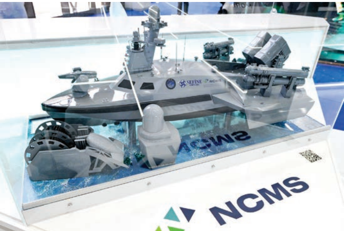
A model of an uncrewed vessel on display at NCMS stand has four stern-mounted anti-submarine torpedo tubes and two box launchers for small surface-to-air missiles
