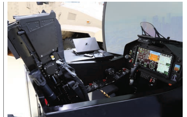
A mock-up of a Calidus B-250 cockpit on display at Saudi's WDS exhibition showed off the L3 Harris tactical mission systems. IMAGE: ALAN WARNES
