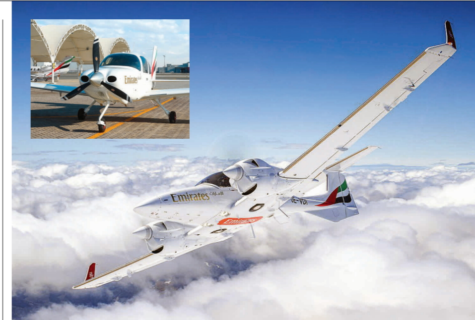
HIGH FLYER: One of EFTA's three new twin-diesel engine Diamond DA-42VI trainers. PICTURE: DIAMOND AIRCRAFT
