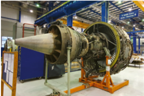
Top: EgyptAir M&E already serves more than 20 African airlines at its Cairo base. Left: El-Khafif (left) signs an agreement with Petra Aerospace of Jordan at MRO Africa. PICTURES: EGYPTAIR M&E. Right: A Trent 700 engine undergoing overhaul at the EgyptAir M&E facility in Cairo. PICTURE: KEITH MWANALUSHI.
