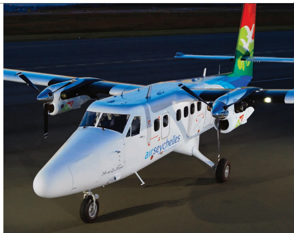
Island hopper: Inter-island sectors in the Seychelles archipelago are served by De Havilland Canada Twin Otter Series 400s.
