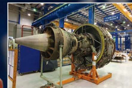
Work under way: A Trent 700 engine undergoing overhaul at the EgyptAir M&E facility in Cairo. PICTURE: KEITH MWANALUSHI
