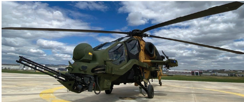
All-round success: The TAI T129 ATAΚ has heavily stepped tandem cockpits, giving both crew the best possible all-round view. PICTURE: TAI.
