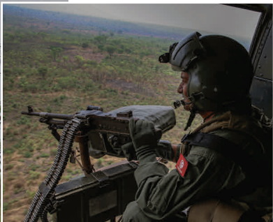
Far left: The Tunisian AB 205s are all armed with cabin-mounted machine-guns. Seen here is an FN MAG, although the Dillon Aero M134D can also be carried. Left: The Tunisian aircraft can operate by day and night, using NVGs, and are able to carry out both close air support sorties using machine guns and rocket launchers, as well as ISR duties thanks to their Star Safire III EO/IR sensor. PICTURES: MINUSCA.
