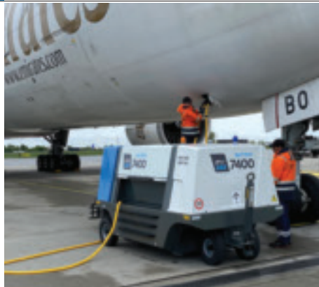
Greener power: ITW GSE's new 140kVA ground power unit (eGPU) supports an Emirates B777-300.
