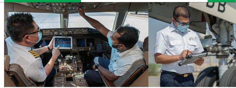
Immediate information: New electronic technical (eTech) logs give Etihad Airways' technicians and flight crew a paperless real-time operational data loop. PICTURES: ETIHAD AIRWAYS.
