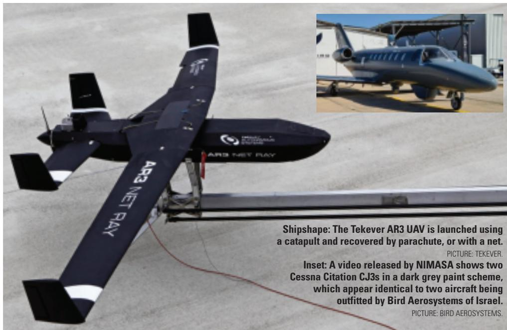
**Shipshape:** The Tekever AR3 UAV is launched using a catapult and recovered by parachute, or with a net.
