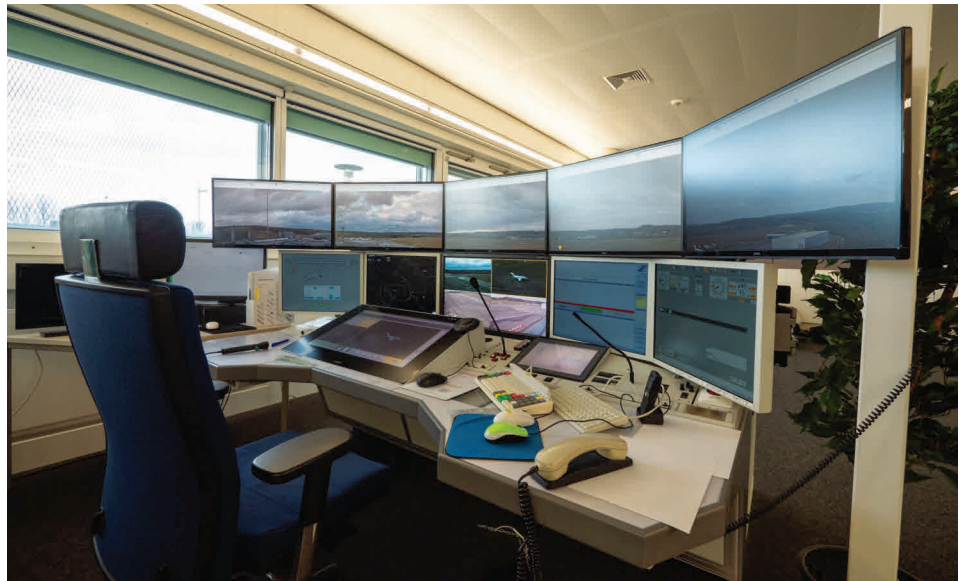
The working station for air traffic control of Saarbrücken Airport in the remote tower centre in Langen. Optimally adapted to the needs of the ATCOs. The entire control environment can be grasped by the controllers at a glance.
