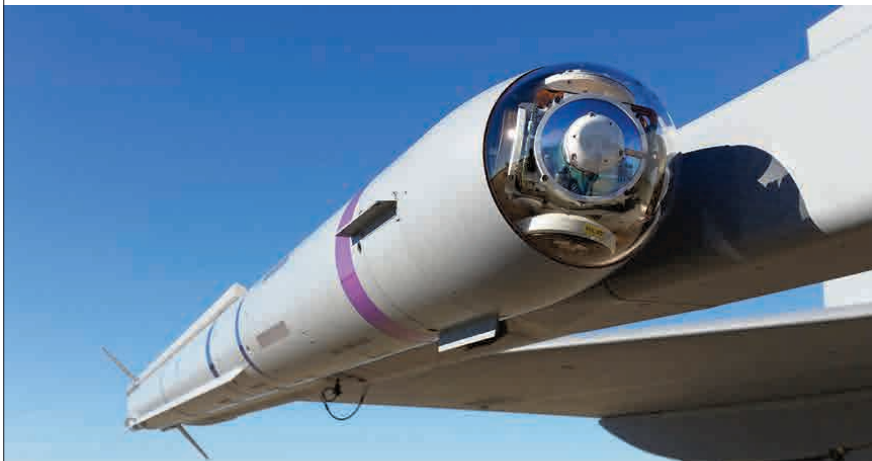
Ready to fire: Denel's A-Darter missile on the wingtip launch rail of a Saab Gripen fighter.
