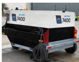
Power-packed: The mobile GPU from manufacturer ITW GSE.
