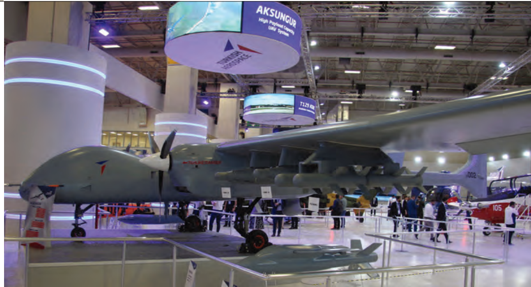
Unveiled: A second Aksungur UAS platform, seen at the Turkish Aerospace stand, was fitted with six hardpoints, with a double rack carrying four laser smart micro munitions.
