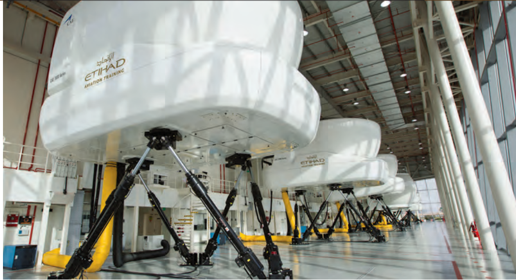
Top-notch: EAT’s facilities are impressive, with no fewer than 11 full flight simulator units, including three Airbus A320 devices, two Airbus A330/A340s, one Airbus A380, two Boeing 777s and three Boeing 787-9s.
