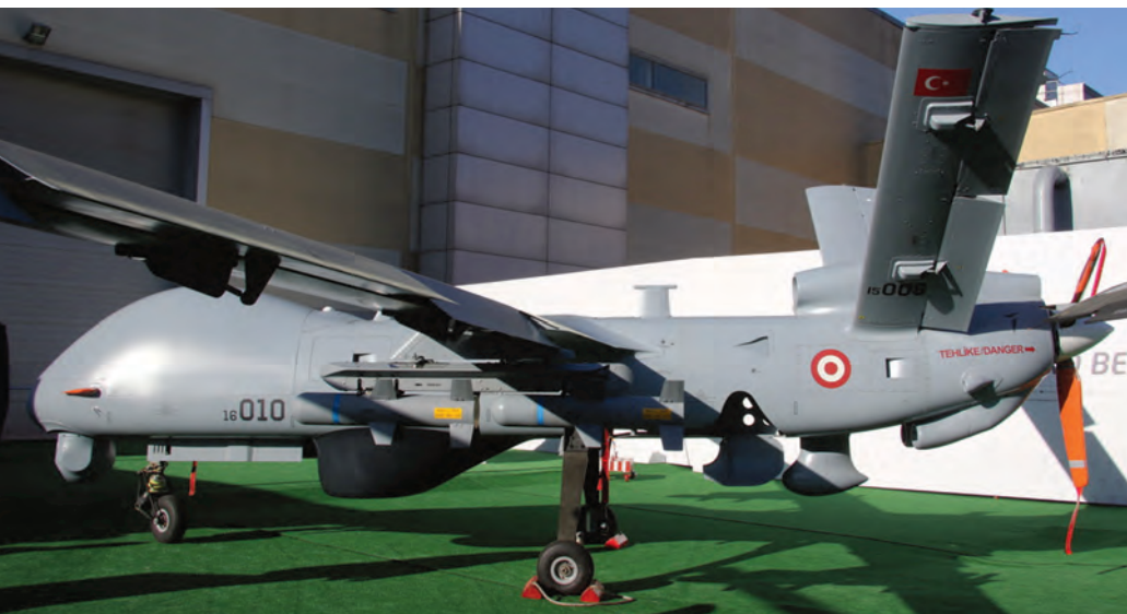
Versatile: The Anka S has a SATCOM inside the nose with a range of 1,000km. This version is used by the navy in the maritime patrol role, although the work has been contracted to Turkish Aerospace. The Land Forces use it as an attack platform.
