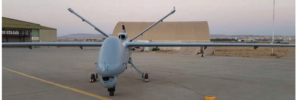
An Anka-S fitted with the indigenous Aselsan CATS system. Below: Turkey's Anka-S UAV is now in service with an indigenous targeting system, and has been cleared to use the MAM-L glide bomb.
