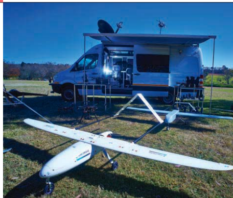
Air Shepherd's fixed-wing UAVs with a mobile ground control station that fly anti-poaching surveillance in Malawi, South Africa and Zimbabwe.
