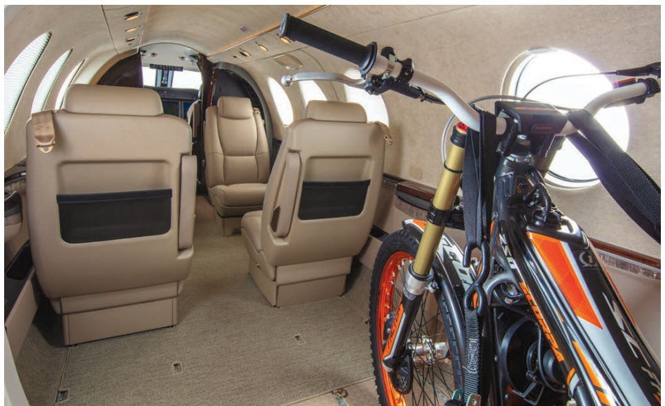
The seats and dividers can easily be reconfigured to take part or all cargo.
