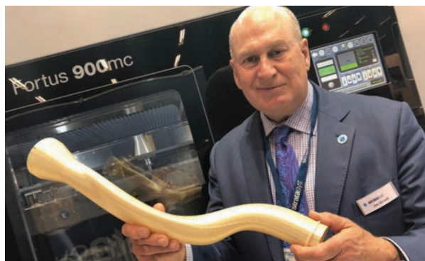
James Orrock holds the new Antero 800NA thermoplastic as he shows off the Fortus 900mc.
