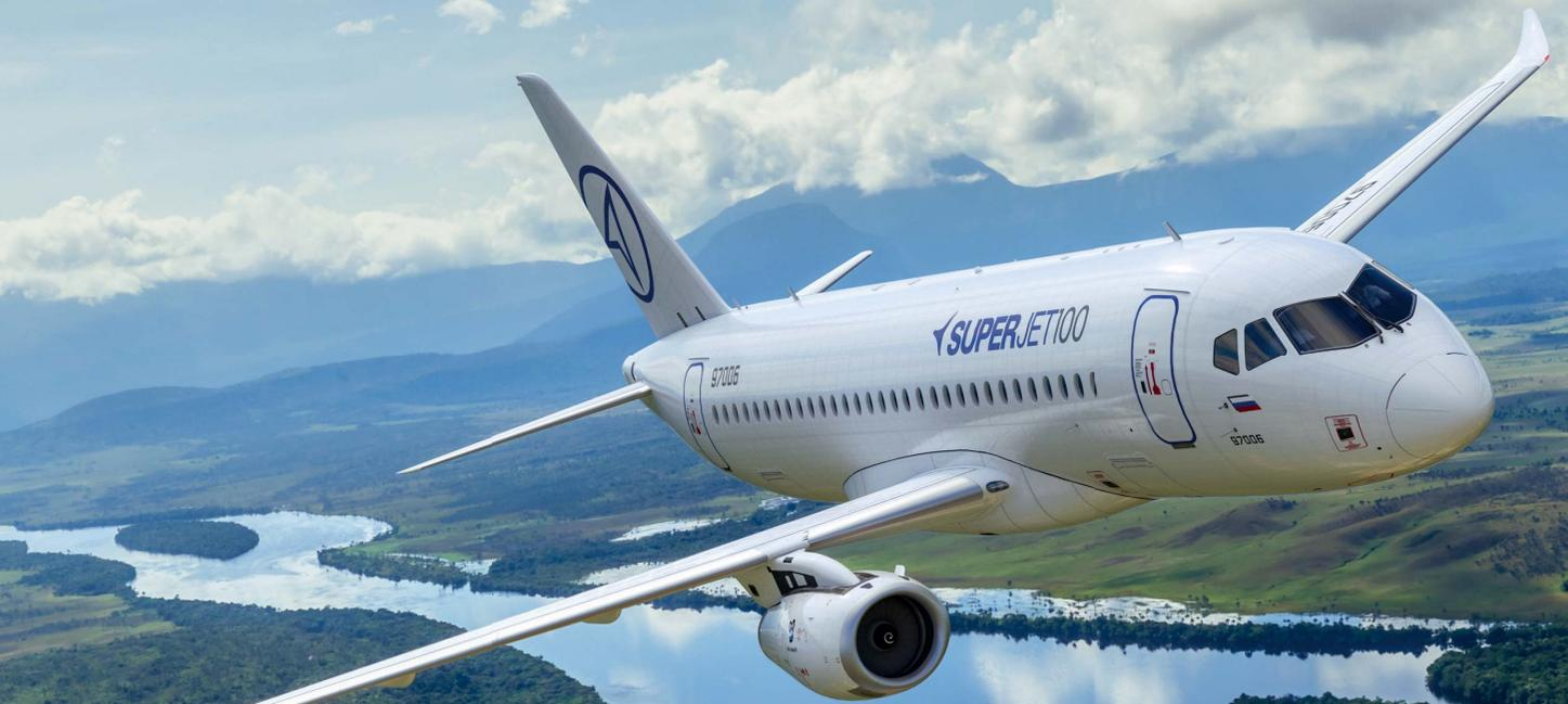
Our new saber-shaped winglets **slash** the air, improving performance and handling especially when operating from short runways with steep approaches. Saberlets also **cut** fuel consumption by at least 3%.
