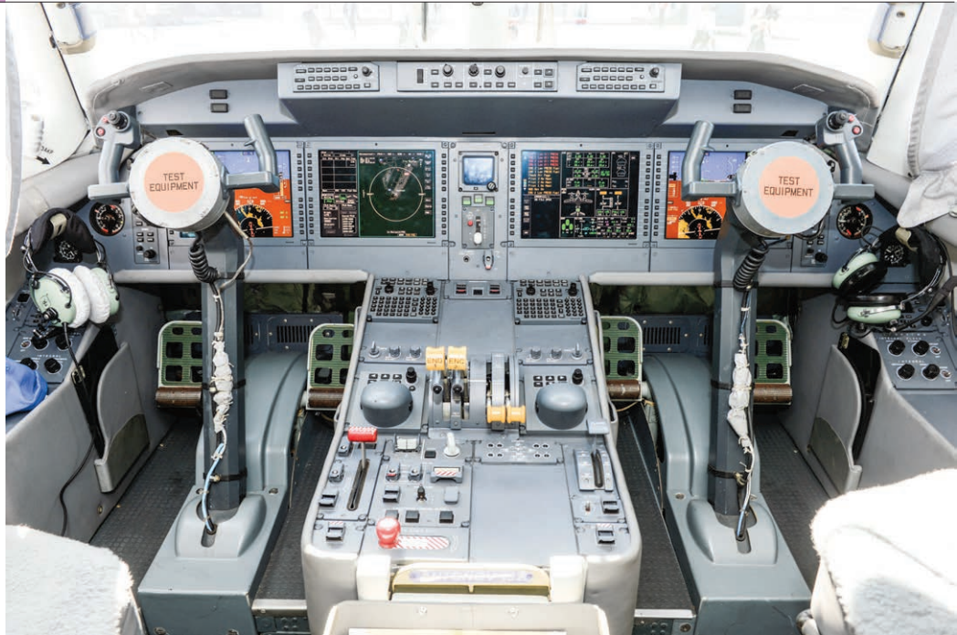
The An-132's Honeywell cockpit is a world away from the An32's analogue displays.
