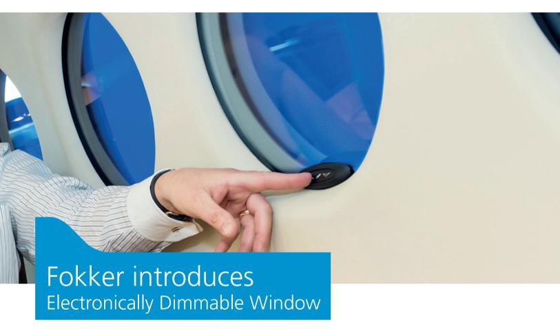
Last year Fokker Services proudly announced the new Electronically Dimmable Window (EDW) concept at the AIX in Hamburg. The innovative EDW is able to block out 99.95% of light coming through, and can generate all types of intermediate dimming modes, such as opaque windows.
