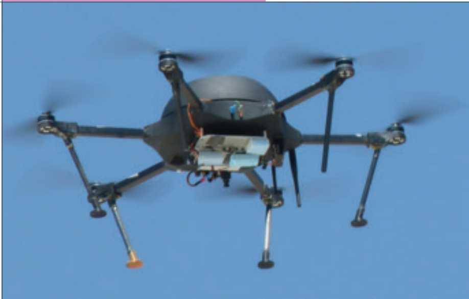
KADDB flew its electric-powered multirole Hexa-Rotor VTOL UAV at SOFEX 2016.
