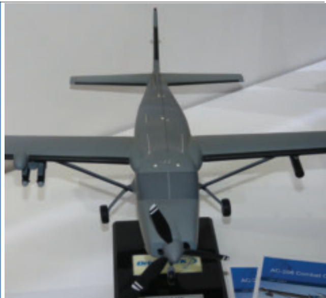
Orbital ATK showed a model of its AC208 Combat Caravan II armed with four Hellfire missiles.
