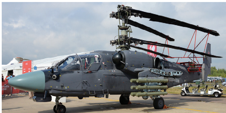
The navalised Ka-52K, seen here in Russian Navy colours, has folding rotor blades and stub wings to save space on board.
