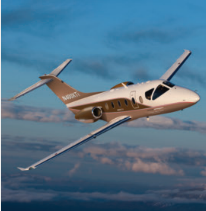
The aircraft is a completely rebuilt Beechjet 400A/XP with Williams FJ44-3AP engines and the Rockwell Collins Pro Line 21 integrated avionics suite.
