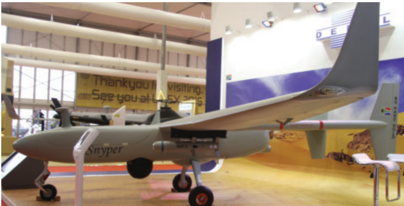
The Denel Sniper is an armed version of the Seeker 400 surveillance UAV and can carry up to four Impi-S missiles, which has evolved from Denel Dynamics' short range Ingwe and Mokopa anti-armour munition.
