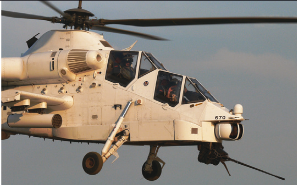
The Rooivalk’s standard armament options during the DRC operations have been its 20mm cannon and pods of 70mm unguided rockets. It was instrumental in disabling the M23 rebel group.
