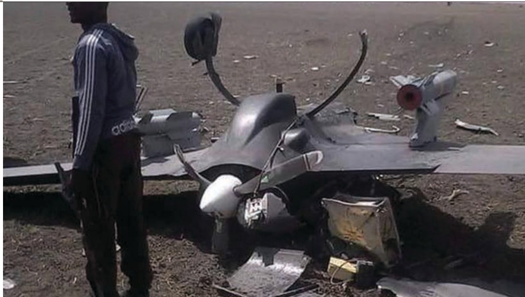
A Chinese-built UAV that crashed in Borno in January. Clearly visible are the sensor turret, air-to-surface missile and lightweight guided bomb.
