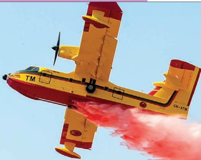
Morocco now has five Bombardier CL415 water bombers to fight wildfires. Right: Some of the RMAF's 20 upgraded F-5E Tigers refuel from a Lockheed Hercules C-130; and below, one of nine of the RMAF's 22 AlphaJets that have been upgraded to LIFT standard.
