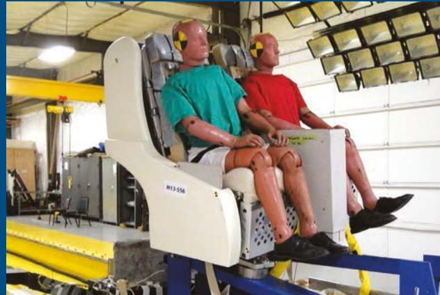
PAC'S 58" PITCH DOUBLE SLEEPER SEAT BEING DYNAMICALLY TESTED FOR FAA CERTIFICATION
