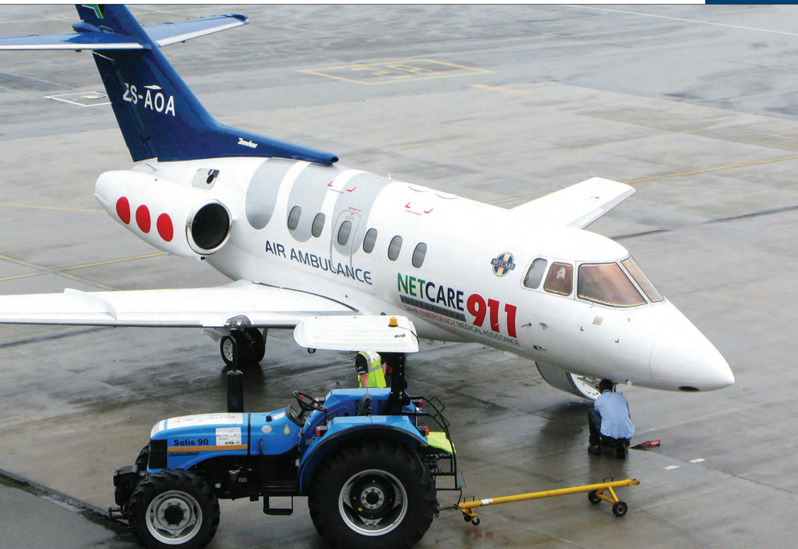
Medair operates a mixed jet fleet that includes this 1990 Hawker 800A. This aircraft will fly from Johannesburg to Lagos non-stop with favourable winds and can carry a pair of Life Port beds and up to three medical personnel. Three flightdeck crew are carried when flight and duty time limits are approached.
