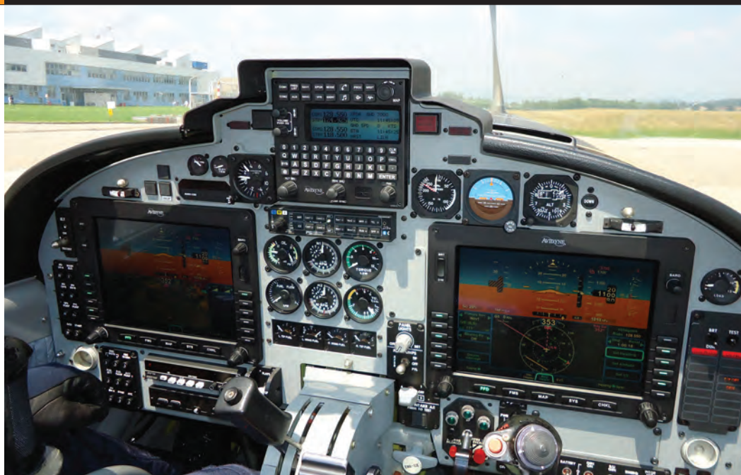
Up-front control (top, centre) and two large multi-function displays – state of the art.
