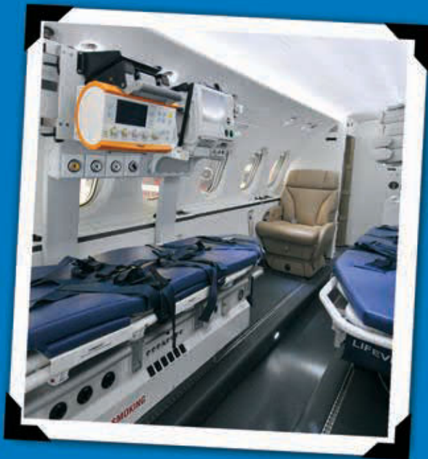
This Hawker 900XP is configured for dual patient transport and is equipped with the latest state-of-the-art medical devices to support almost any medical condition, including neonatal transport. The new carbon fiber components increase strength and lower system weights with unlimited functional design options.
