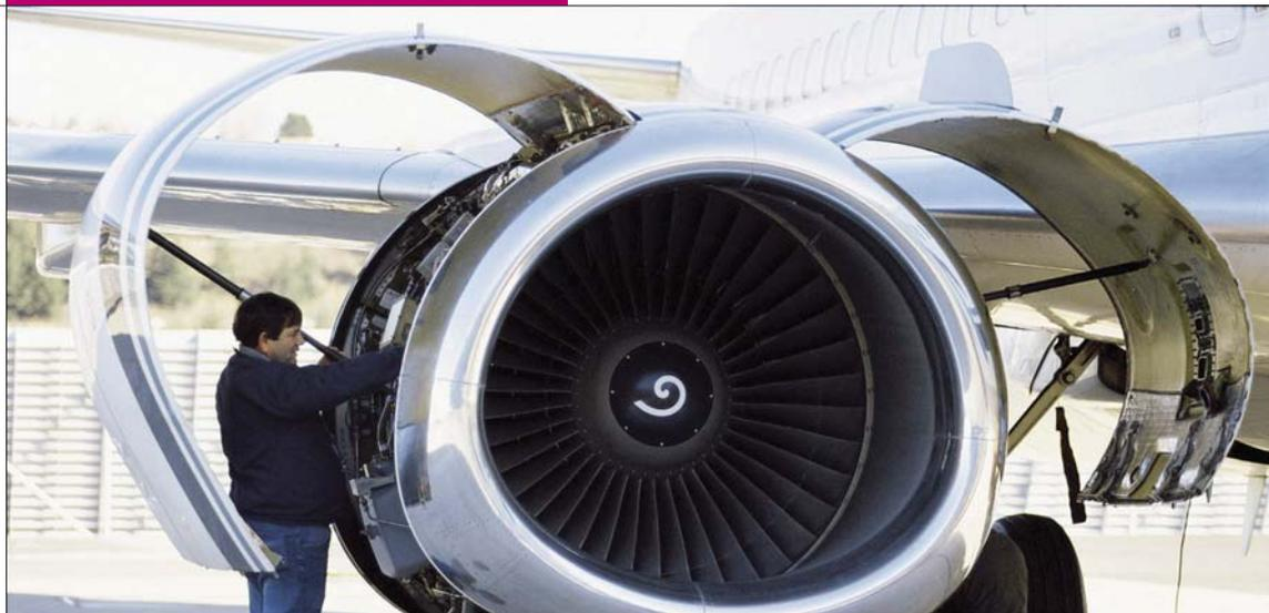
This CFM56-3C on a Boeing 737 is being prepared for an on-wing core upgrade.
