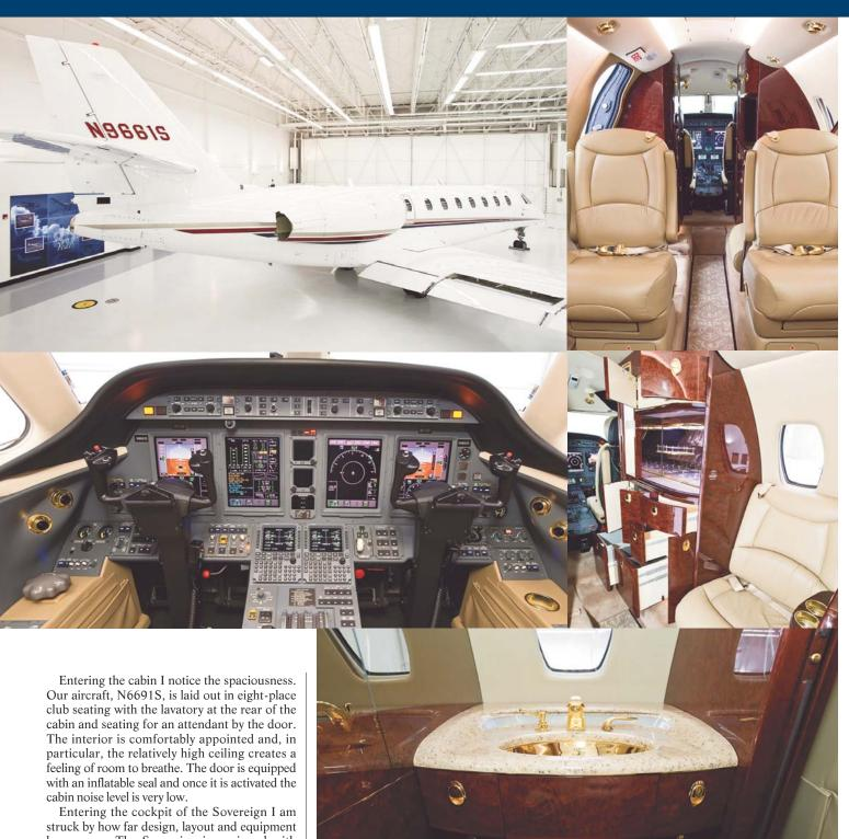
Entering the cockpit of the Sovereign I am struck by how far design, layout and equipment have come. The Sovereign is equipped with Honeywell Epic Avionics, and a lot of thought and planning has been employed. The primary flight displays are large, easy to see and interpret. The engines have FADEC control and, as opposed to round gauges, have bar indicators and are comfortable to use.
