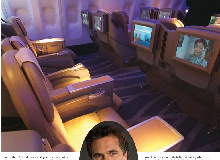
and other MP3 devices and play the content on the screen. In premium economy Thales i-2000 broadcast system delivers six channels of audio to each of 96 seats and video to overhead dropdown screens. There are two laptop power sockets for every three seats.
